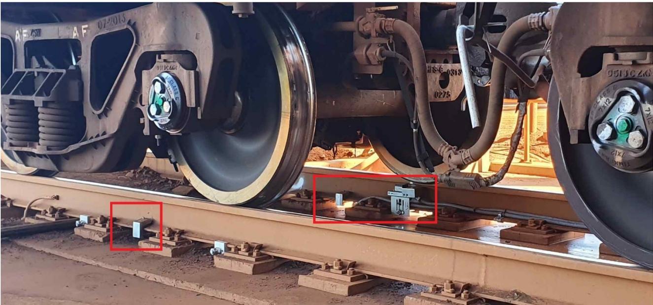
Figure 4: Loadcell and track switch installation
